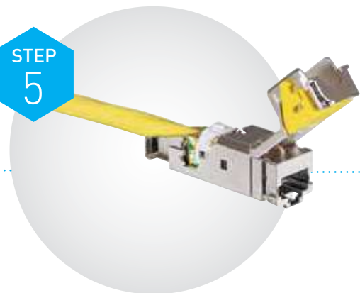
Install the wire housing without pushing
