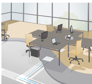
Screed floor system
