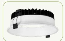
Ceiling cutout: Ø 110 mm, height 50 mm for 12 W /15 W. Ø 14 5mm , height 55 mm for 18 W .Ø 165 mm , height 55 mm for 24 W.
